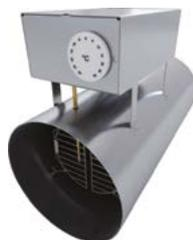
Also the heater has two protection thermostats and a perforated metal filter which can easily be maintained via the inspection door. This significantly increases its life span especially when the heater is installed on the outdoor air side for frost protection purposes. Alternatively it can be used as post-heater to achieve the required indoor air temperature.
